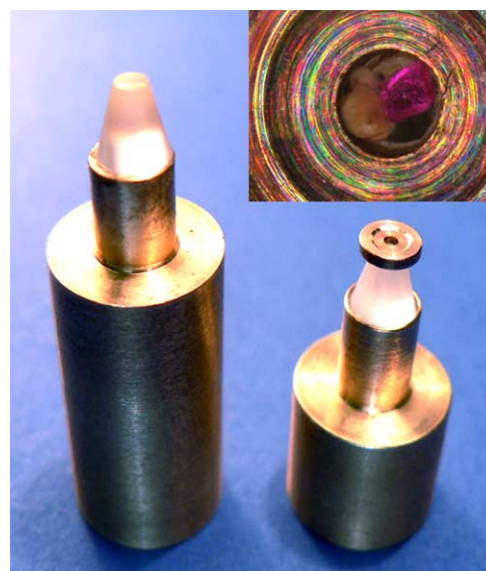
Fig. 6. The pistons of the SAC assembled with sapphire anvils. The lower sapphire anvil is assembled with the gasket. Inset: blow-up of the 0.5 mm sample hole in the gasket. The small speck of DPPH (wrapped up in a flake of PTFE tape) is shown adjacent to the crystal of ruby.
